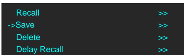
3. Turn the rotary knob, and select the location that need to save, push the rotary knob to confirm.
