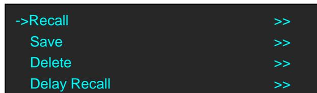
3. The button on is ready for recall, and button flashes means just recall. Push the button on or turn the rotary knob to select the location that need to recall, push the rotary knob to confirm.
